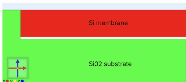
Simple CMUT structure showing cross section (top) and cutaway of unit cell pattern (bottom)
