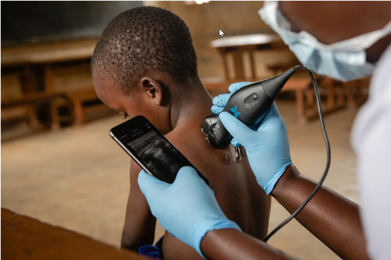
Butterfly Network developed a handheld ultrasound machine using capacitive micromachined ultrasonic transducer (CMUT) technology. BUTTERFLY
